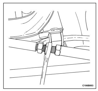
4. Hold the adjustment screw and tighten the toe adjusting screw jam nut.
