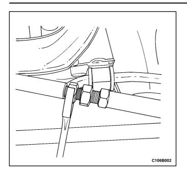
3. Turn the adjustment screw until the preferred rear toe specification is obtained. Refer to \(\text{\text{Wheel}}\) Alignment Specifications" in this section.
